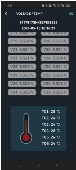
Figure 26: Battery pack voltage & temperature information in real time
