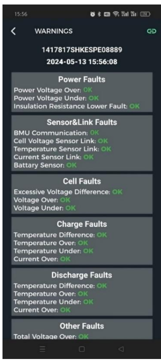
Figure 25: Battery pack real-time alarm
